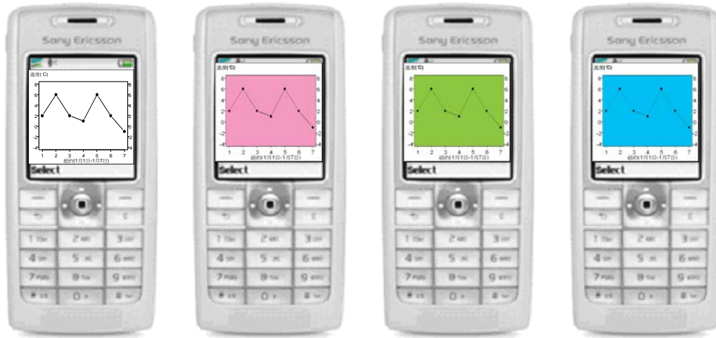
Figure 2 Background colors of line graphs based on color combinations of (R,G,B) / (H,S,B) from left to right: (255,255,255)/(0,0,100), (172,211,115)/(85,46,83), (0,191, 243)/(193, 100,95), and (244, 154,193)/(334,37,96).
