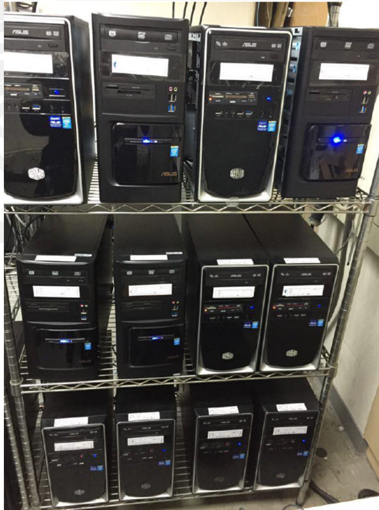
FIGURE 4.1: Spark and Hadoop Computing cluster
