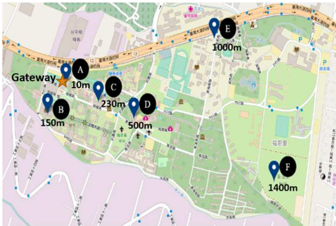
FIGURE 4.8: LoRa Campus Test Chart
