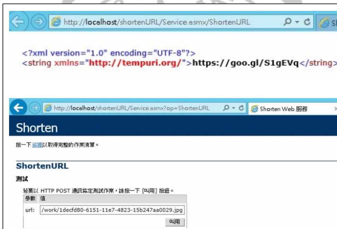
Figure 4: The self-developed Google-URL-Shortener Service. The full URL is http://ecgtif.vghtc.gov.tw/work/1decfd80-6151-11e7-4823-15b247aa0029.jpg (Only the right portion is shown due to long string). The returned result is in xml and the shortened URL is https://goo.gl/S1gEVq (See the right string on the top rectangle).
