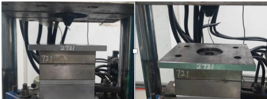
Figure 3.8 Change injection port to cylindrical shape
