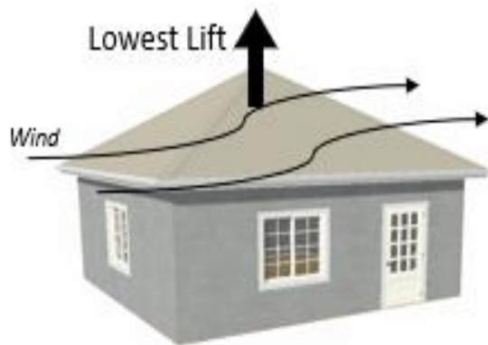
C. Pyramid roofs gets the lowest uplift
