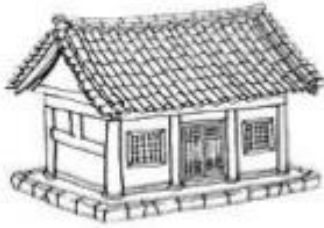
matbae (gable) roof
