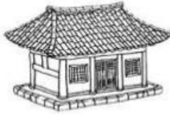
ujingak (hipped) roof
