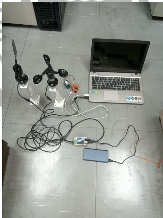
Figure 3. An air box, i.e., an IoT node, consists of a dust sensor, a wind-speed sensor and a wind-direction sensor all connecting to an Arduino.
