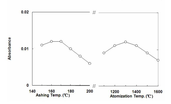
Fig. 1 Effect of the ashing and atomization temperatures on the absorbance of Hg for 0.46 ng Hg in 50  $\mu$ L of concentrated methanol solution.
