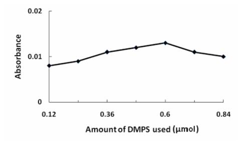
Fig. 4 Effect of the amount of DMPS on the absorbance of Hg for 0.48 ng Hg in 50  $\mu$ L of concentrated methanol solution.
