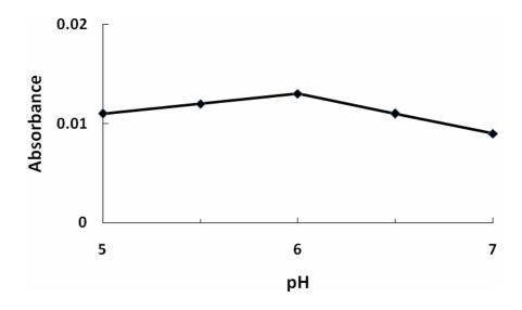
Fig. 5 Effect of pH of sodium acetate buffer on the absorbance of Hg for 0.48 ng in 50  $\mu$ L of concentrated methanol solution.
