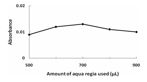
Fig. 2 Effect of the amount of aqua regia on the absorbance of Hg for 0.48 ng Hg in 50  $\mu$ L of concentrated methanol solution.
