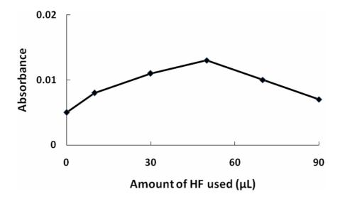
Fig. 3 Effect of the amount of HF on the absorbance of Hg for 0.48 ng Hg in 50  $\mu$ L of concentrated methanol solution.
