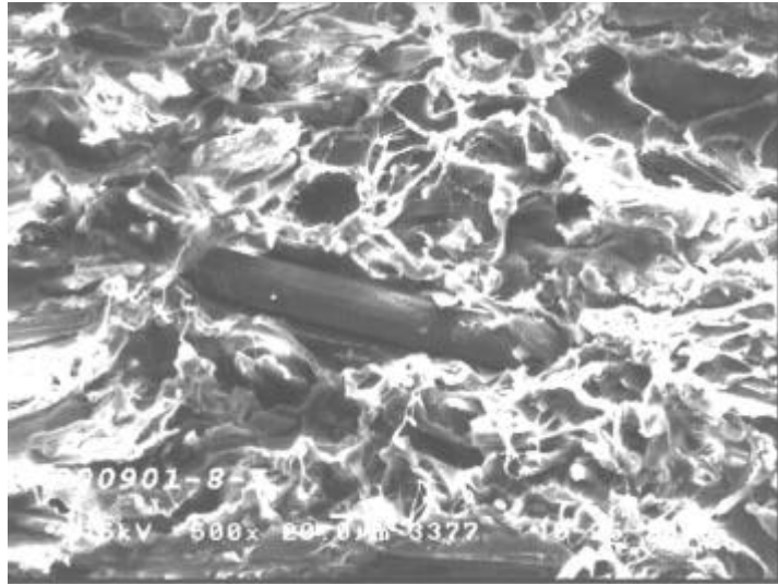
Figure 5.6(a) SEM micrographs of fracture surface of notched impact specimens for unmodified composite.
