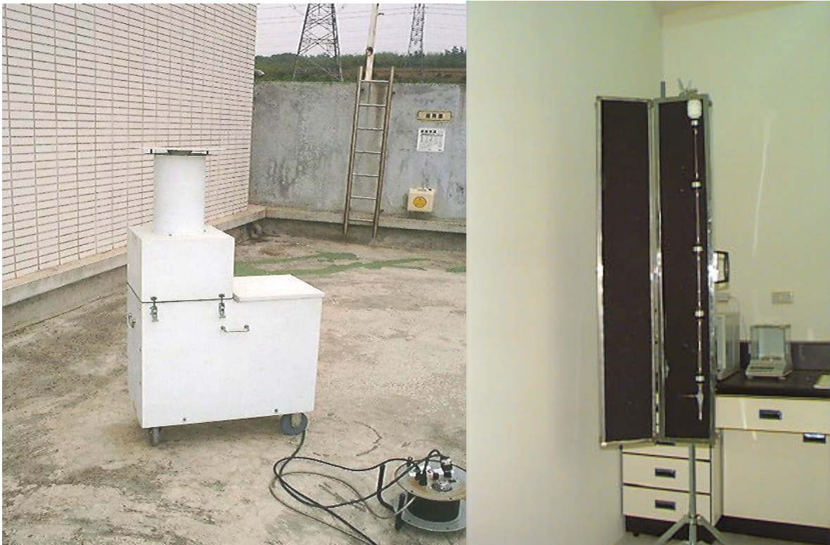
Figure 3.3-2. The outward appearance of the Universal sampler (left) and ADS (right).
