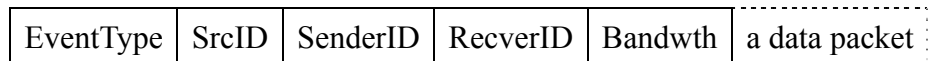
Figure 3. Extra fields of a piggybacked packet as the first or the last packet of an event
