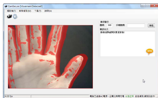
Fig.2 Area of difference is marked in red, where misjudgment of motion occurs due to noises
