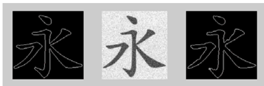
(a)書法字型掃描檔 (b)灰階影像檔 (c)灰預測邊緣偵測
