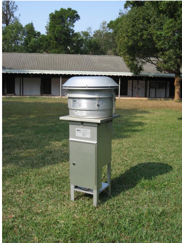
Figure 2-3. PM 10 high volume air sampler, Tisch Environmental, Inc., TE-6070 High Volume MFC.
