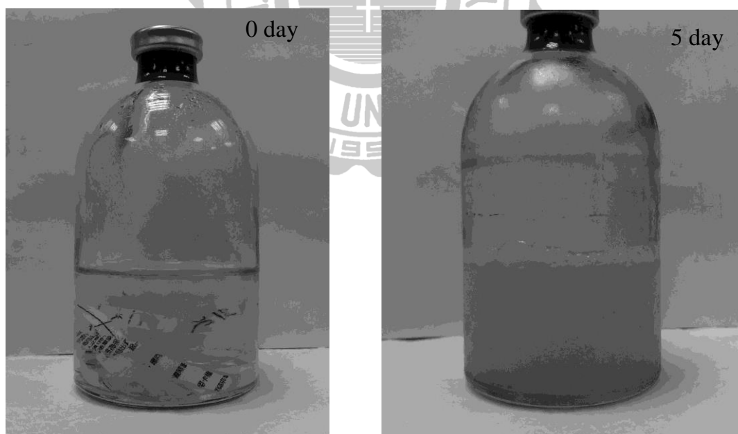
Fig 4-2 Biodegradation of waste paper by thermophilic anaerobic microorganisms from rumen fluid.
