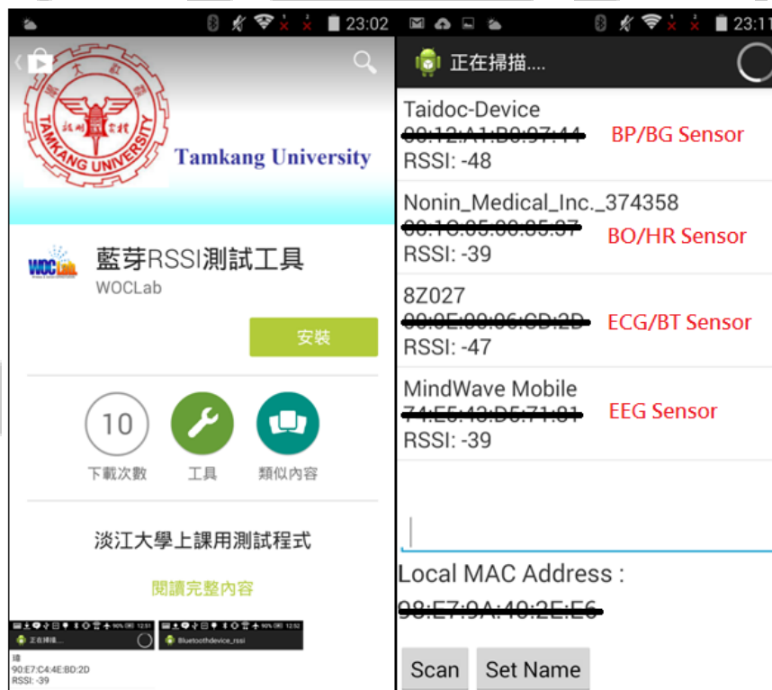
Figure 16. The measurement results on Bluetooth radio radiation of different physiological sensors by using the tool for Bluetooth RSSI measurement which is an APP developed by Tamkang University, Taiwan.
