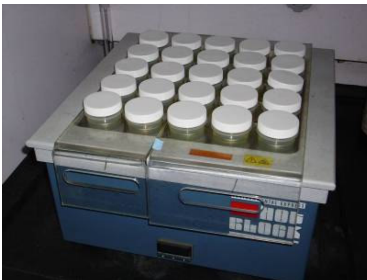
Fig.3.5 Flat platform heater (Hot Block Model SC 150, USA).
