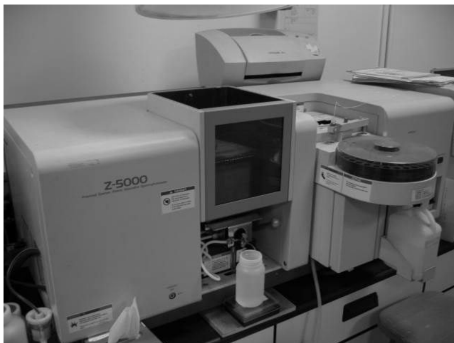
Fig.3.6 Polarized-Zeeman Atomic Absorption Spectrophotometer (Z-5000, Hitachi, Japan). It is comprised of two parts : Flame Atomic Absorption Spectrometry (FAAS), and Graphite Furnace Atomic Absorption Spectrometer (GFAAS).
