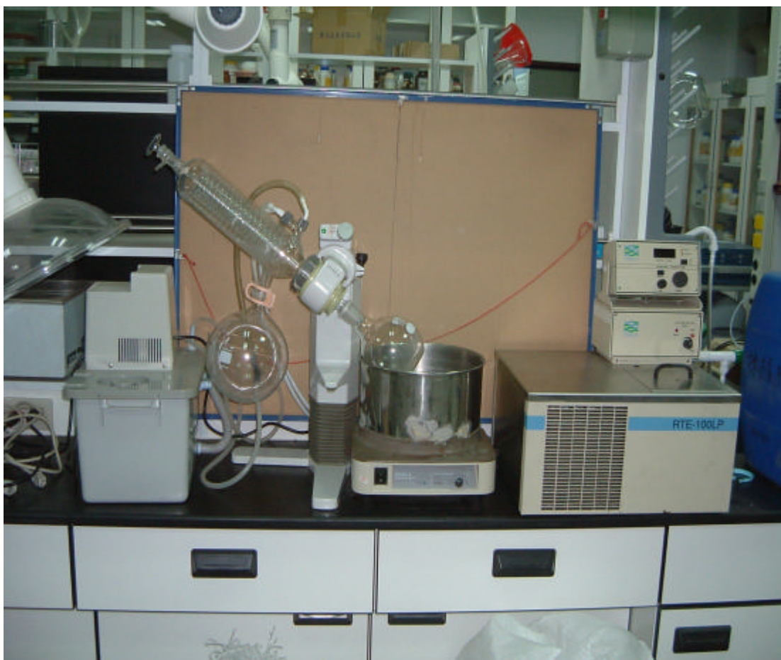
Figure 3.4-4. The structure of rotary evaporator for concentrated process.
