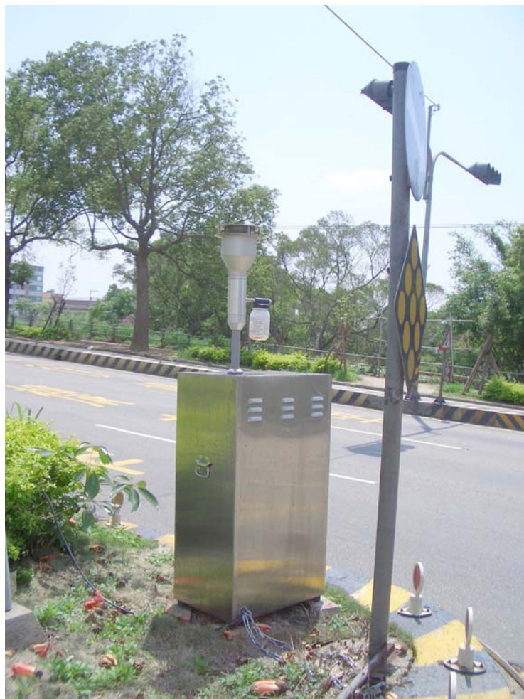
Fig. 3.2-1 The structure of versatile air pollutant system used for fine and coarse particulates collection.
