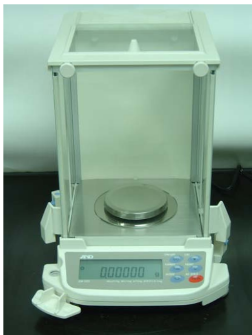
Fig. 3.2-2 The illustration of analytical balance (AND GR-202) used for particle mass measurement.
