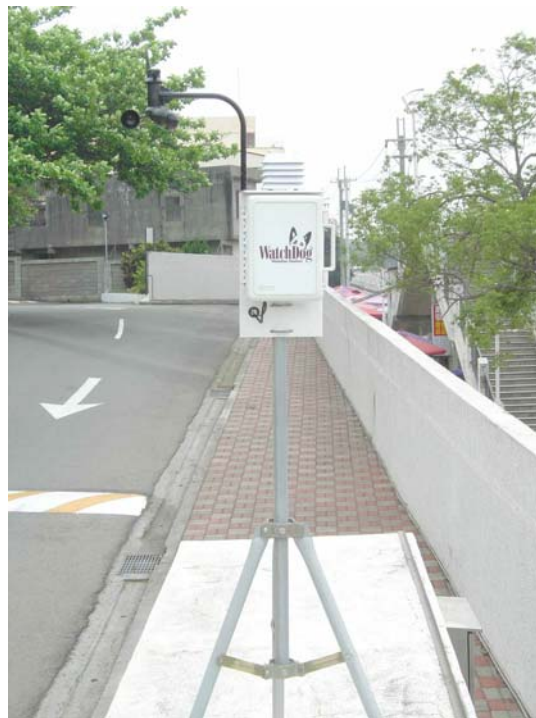
Fig. 3.3-2 The illustration of portable weather station (Watchdog model 525) used for record wind speed and wind direction.
