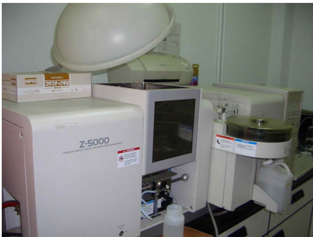
Fig. 3.2-3 The structure of Z-5000 flame atomic absorption spectrophotometer used to measure the metallic element concentrations.
